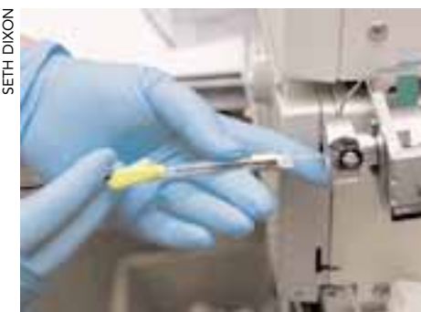
Individualized dosing was used for each child who received topotecan as part of SJMB96. Here, a technologist in the laboratory of Clinton Stewart, PharmD, injects an extract of the patient’s plasma into a machine that tells how much topotecan is in the patient’s body.
